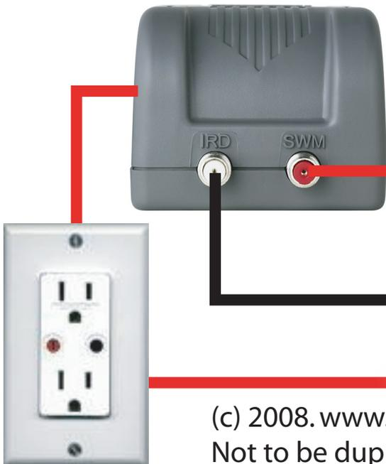
NOTE: Connect only one line to the HR20/HR21 SWM/FTM/SAT1 port. Do not use B-Band converters and connect nothing to the SAT2 port.
